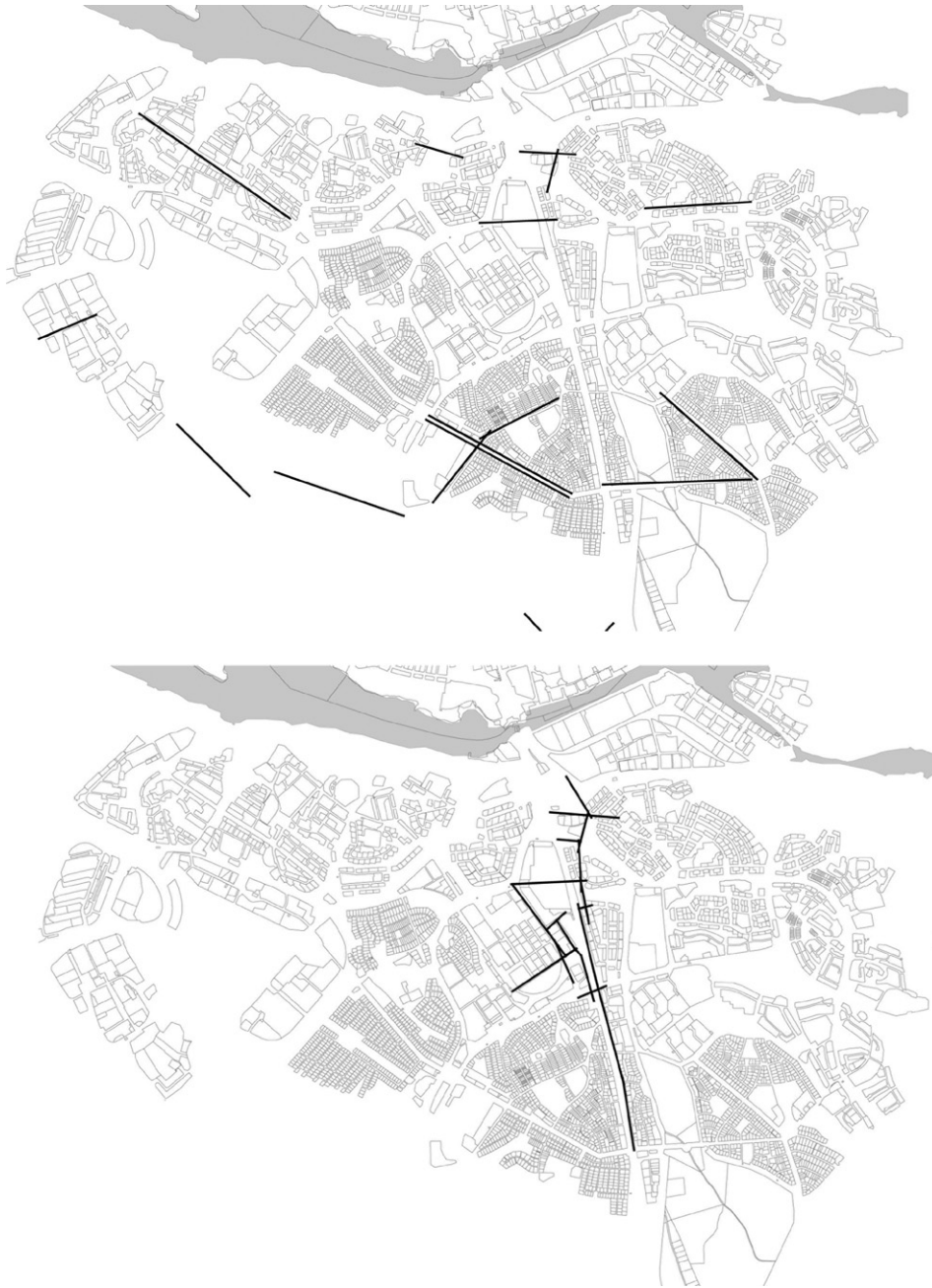
Fig. 27. The most integrated lines in an area of the southern suburbs of Stockholm. Local integration (top) and global integration (bottom).
