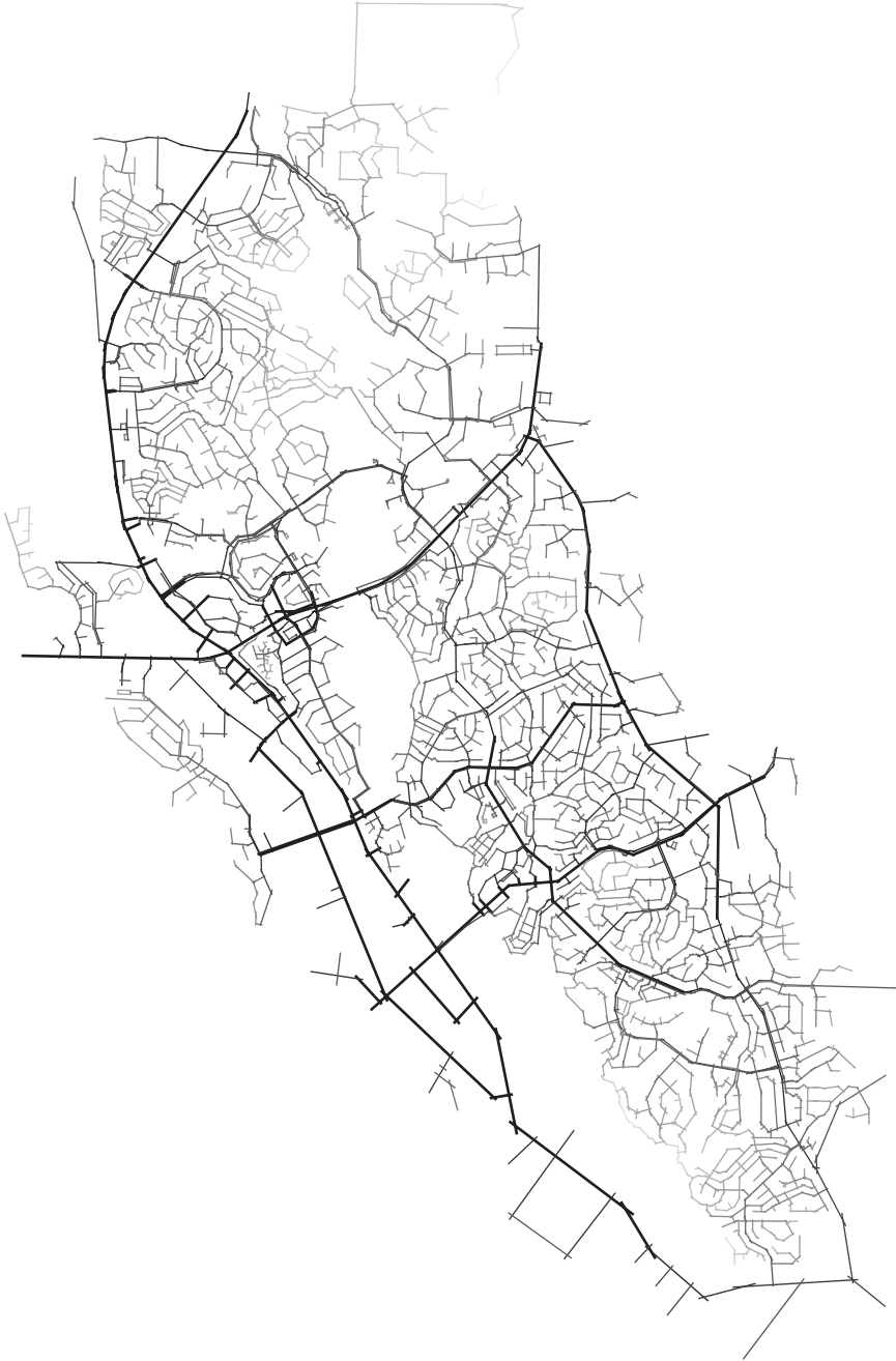
Fig. 35. Map D: fractional axial analysis of the combined cart path and road system.
