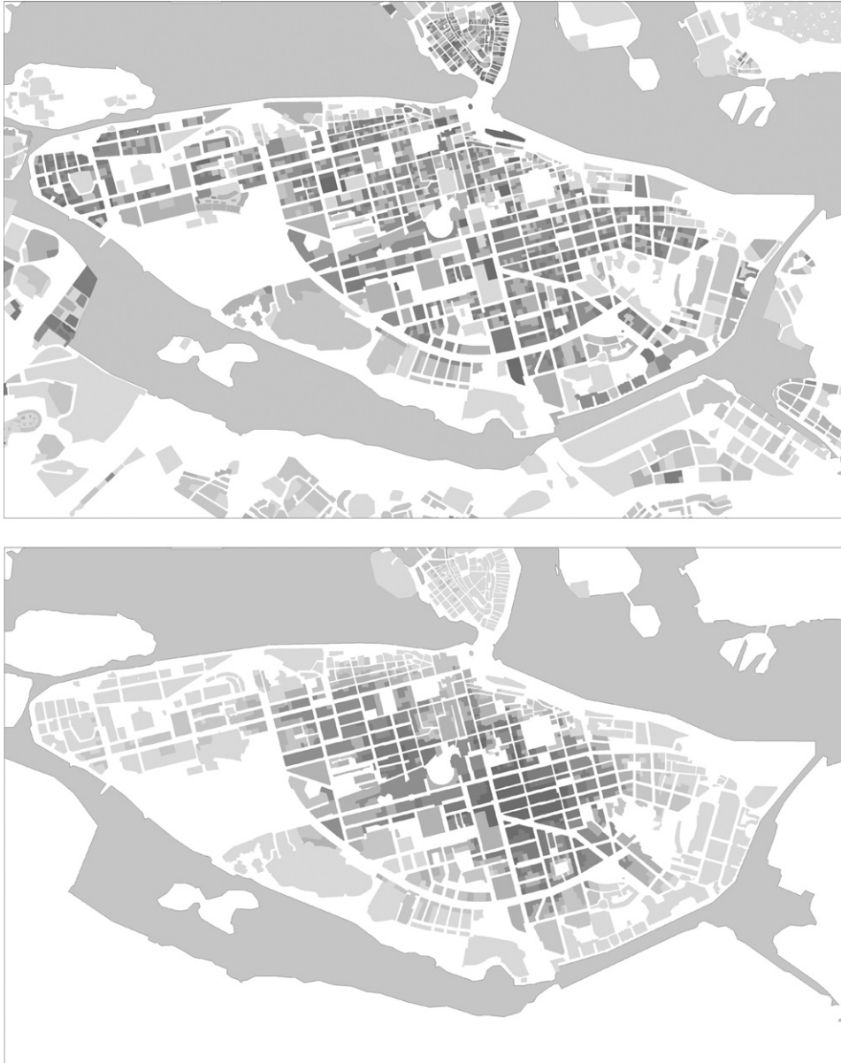
Fig. 28. Geographical data on population represented as densities within geographical units – in this case plots – for an inner city area of Stockholm (top). Geographical data on population represented as accessible population within a radius ( r = 700 m) from each plot, following the actual street-pattern, for the same area (bottom).
