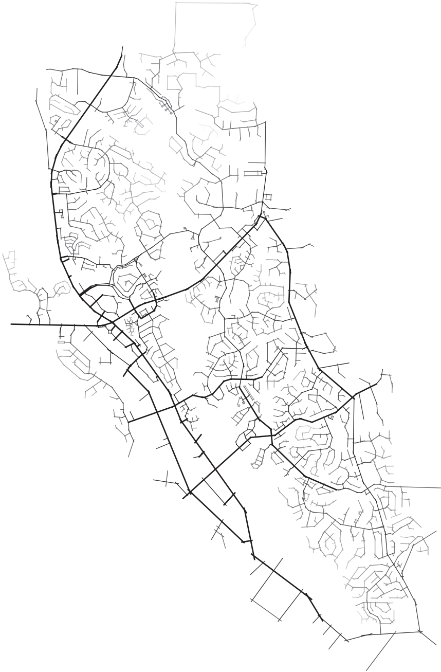
Fig. 34. Map C: fractional axial analysis of the road system.
